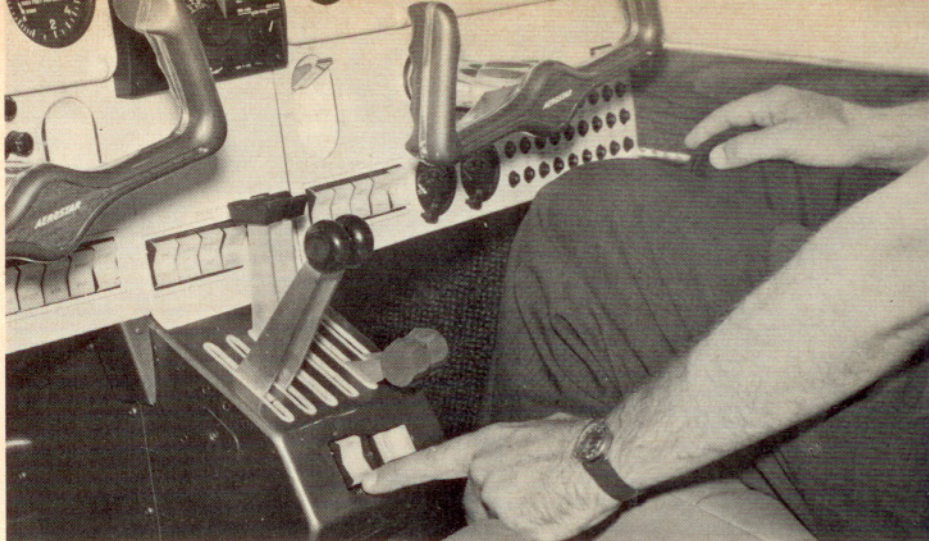
Trim in Aerostar 320 is controlled by electrical tab on throttle quadrant. Rollout model of the Ted Smith line has numerous such switches for various functions, including nosewheel steering
