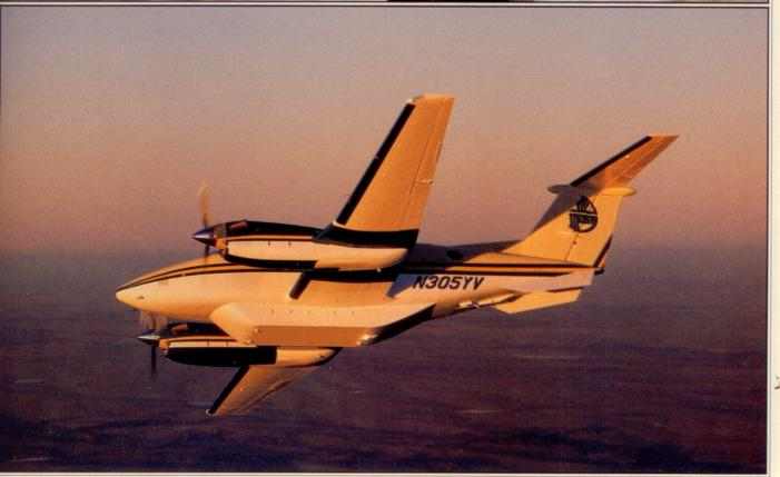
the airplane a lot. The 1300 will, at maximum cruise power, do 270 knots at 22,000 feet, only a few knots slower than a 200 and actually faster than the 1900. The 1300 is restricted to 25,000 feet (the 200 is certified to 35,000 feet) because of an additional emergency oxygen requirement above 25,000 feet.
