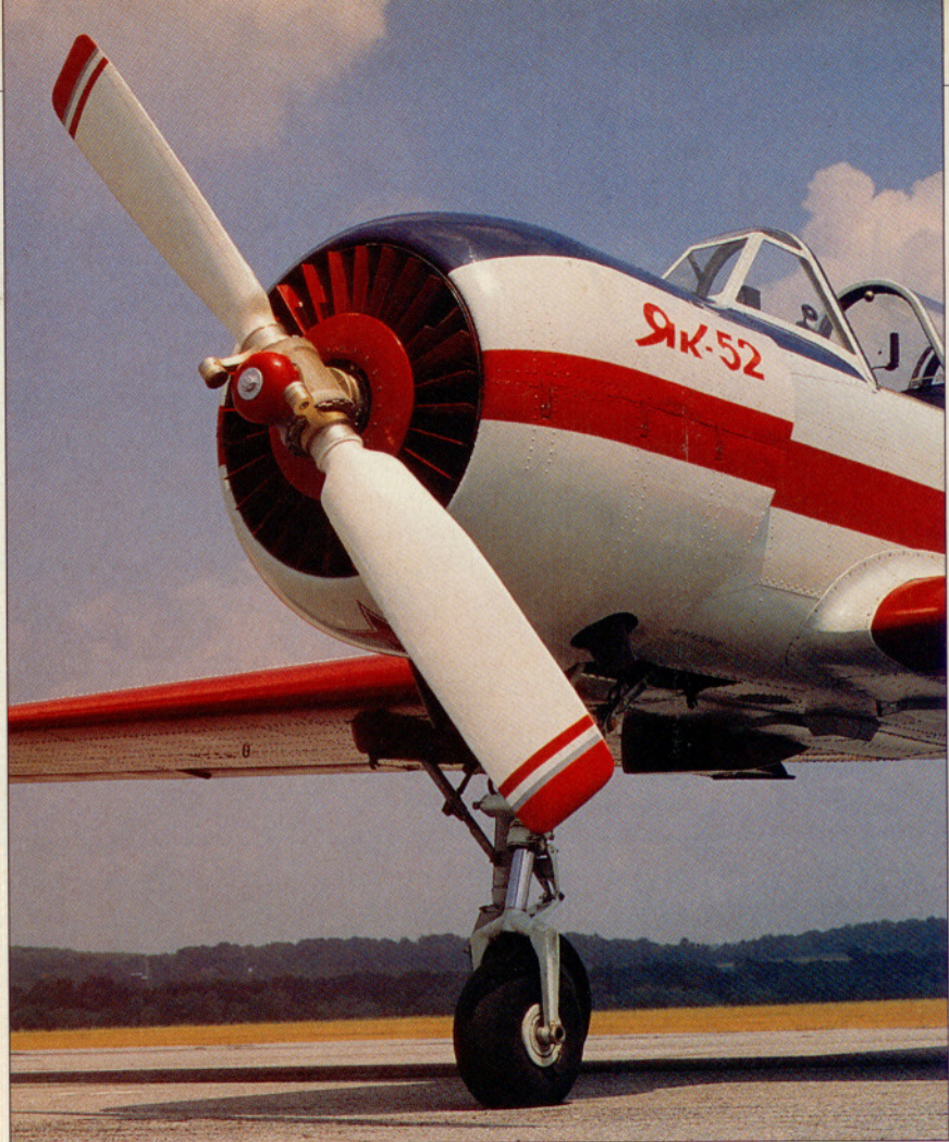
The huge wooden propeller requires tall landing gear to provide ground clearance. There are attachments under the left wing root for a stepladder, although it is not included with used aircraft.
