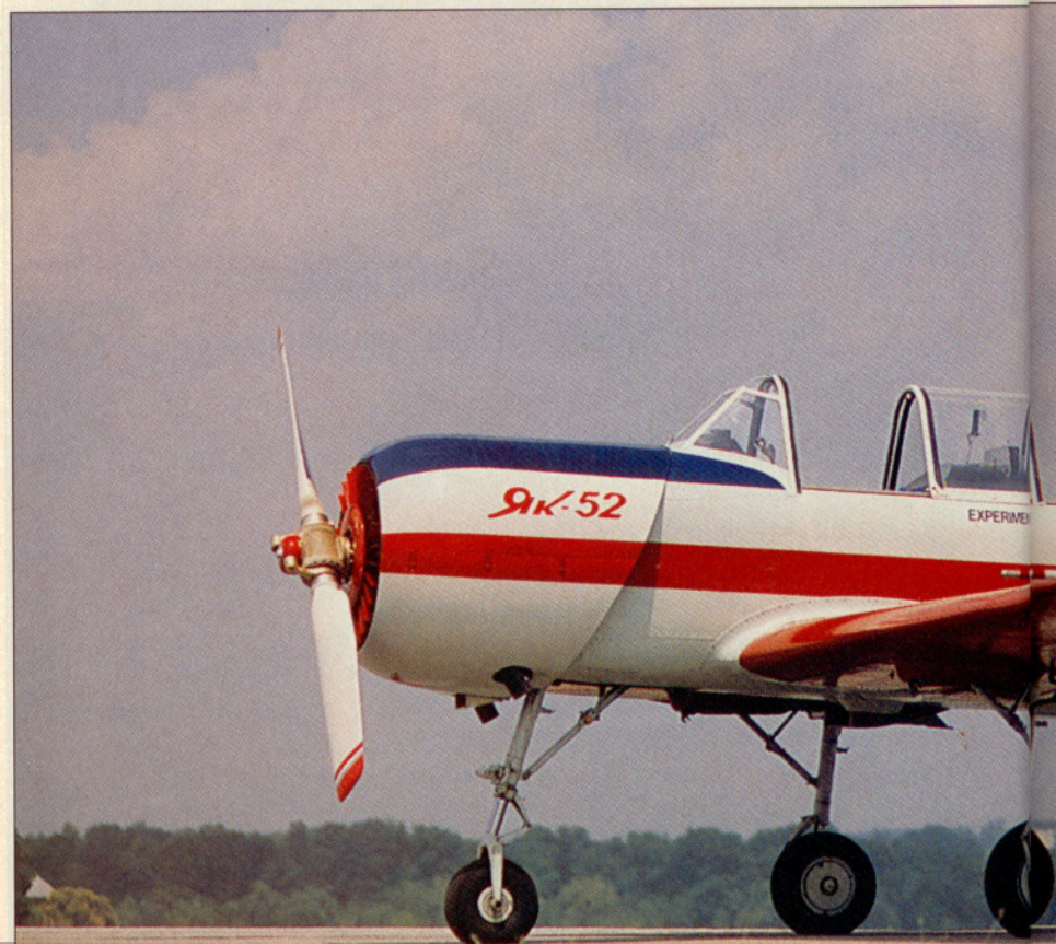
The huge wooden propeller requires tall landing gear to provide ground clearance. There are attachments under the left wing root for a stepladder, although it is not included with used aircraft.
